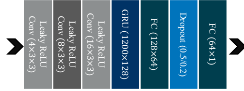
Fig. 10. Flow rate estimator architecture.
